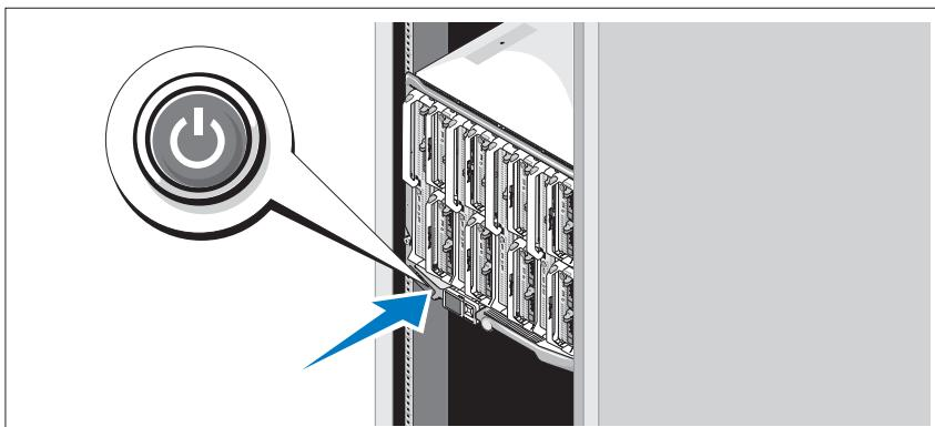
Press the power button on the enclosure. The power indicator should light.
