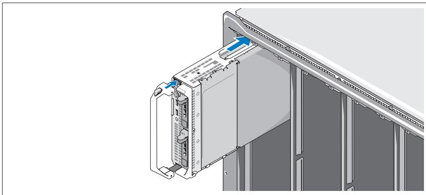
Beginning at the top, slide the modules into the enclosure from left to right. When the blade is securely installed, the handle returns to the closed position.
